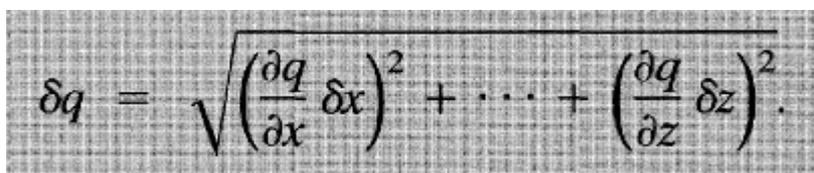
$$\delta q = \sqrt{\left(\frac{\partial q}{\partial x} \delta x\right)^2 + \dots + \left(\frac{\partial q}{\partial z} \delta z\right)^2}$$
