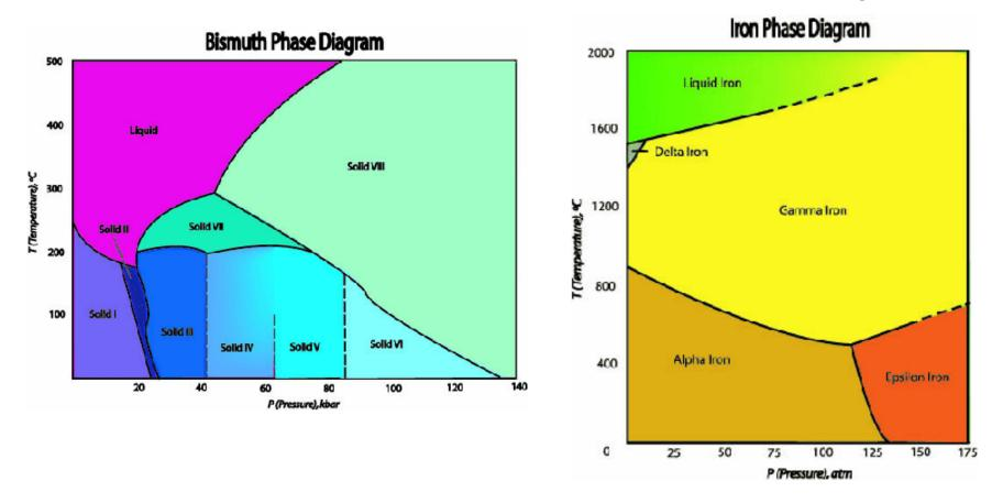
Bi (and Sb) has a similar solid-liquid volume anomaly to H<sub>2</sub>O
