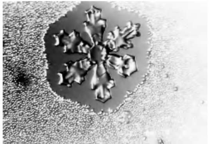
Fig. 6.36 Laboratory demonstration of the growth of an ice crystal at the expense of surrounding supercooled water drops. [Photograph courtesy of Richard L. Pitter.]
